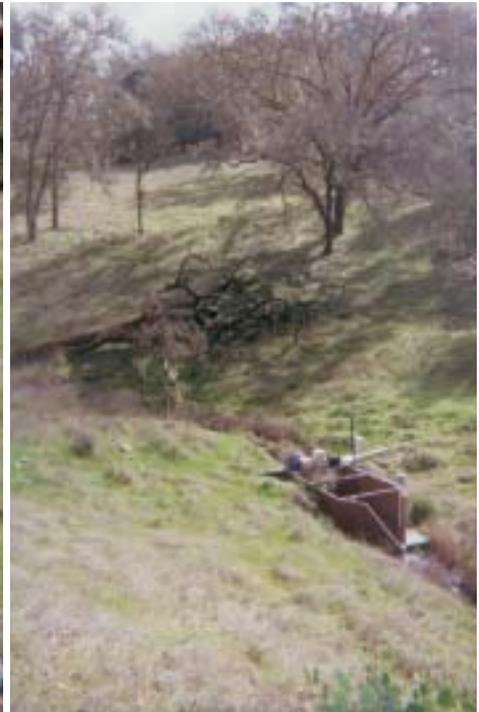
Stream flow and water-quality sampling equipment are located at the outlet of each experimental watershed. In coming years, studies will focus on the roles that grazing and fire management play in plant communities, hydrology and water quality.
